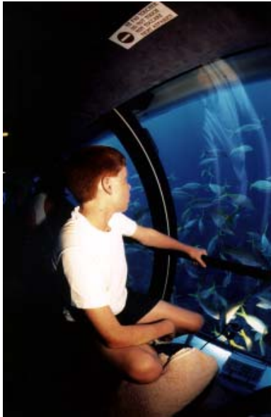
Passenger compartments composed of transparent acrylic provide exceptional viewing and characterize several U.S. Submarines' designs.
