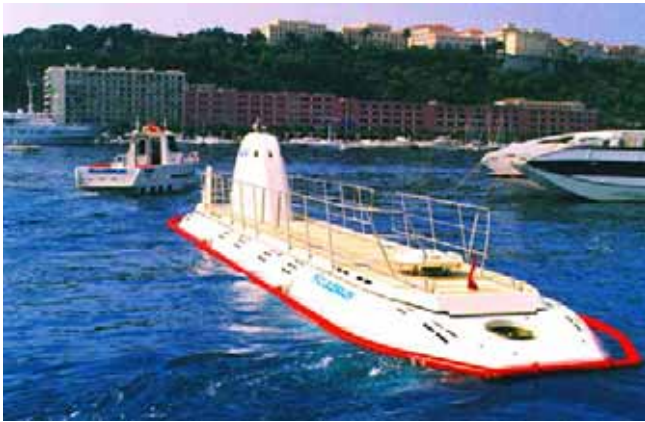
The Deepstar submarine on the surface. The submarine has made 3200 problem-free dives and is 20 meters in length and weighs 92 tons.
