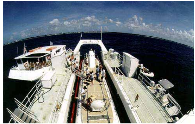
The complete equipment group shows the Deepstar submarine docked in the support barge with the catamaran alongside.
