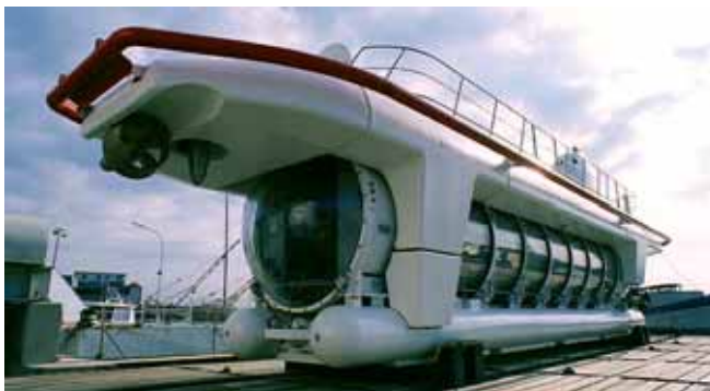
The unique Deepstar submarine with its transparent hull.
