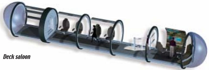
Deck saloon is composed of transparent acrylic cylinders
