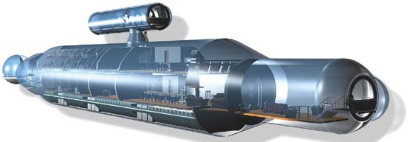
The steel pressure hull of the Phoenix contains the three decks and various internal spaces and is penetrated by viewport forgings and entrance hatches as well as penetrator plates through which electrical, hydraulic and pneumatic connections pass externally.
